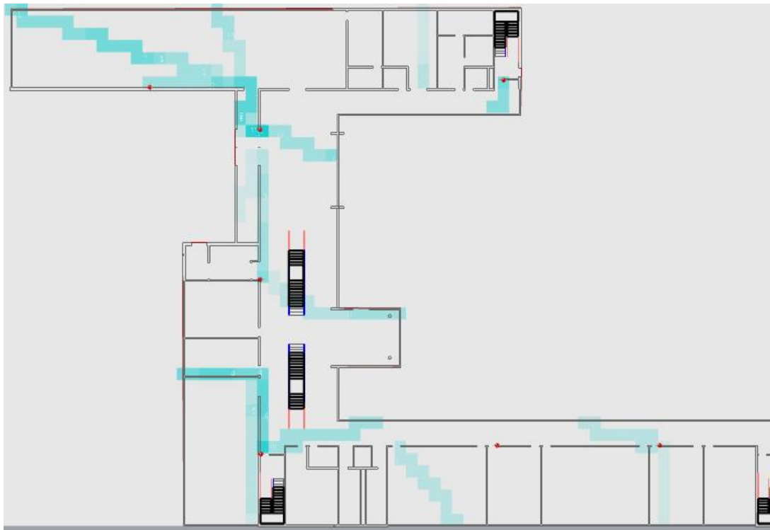
Figure 8. Heatmap of the con-fire safety planning Simulation.
