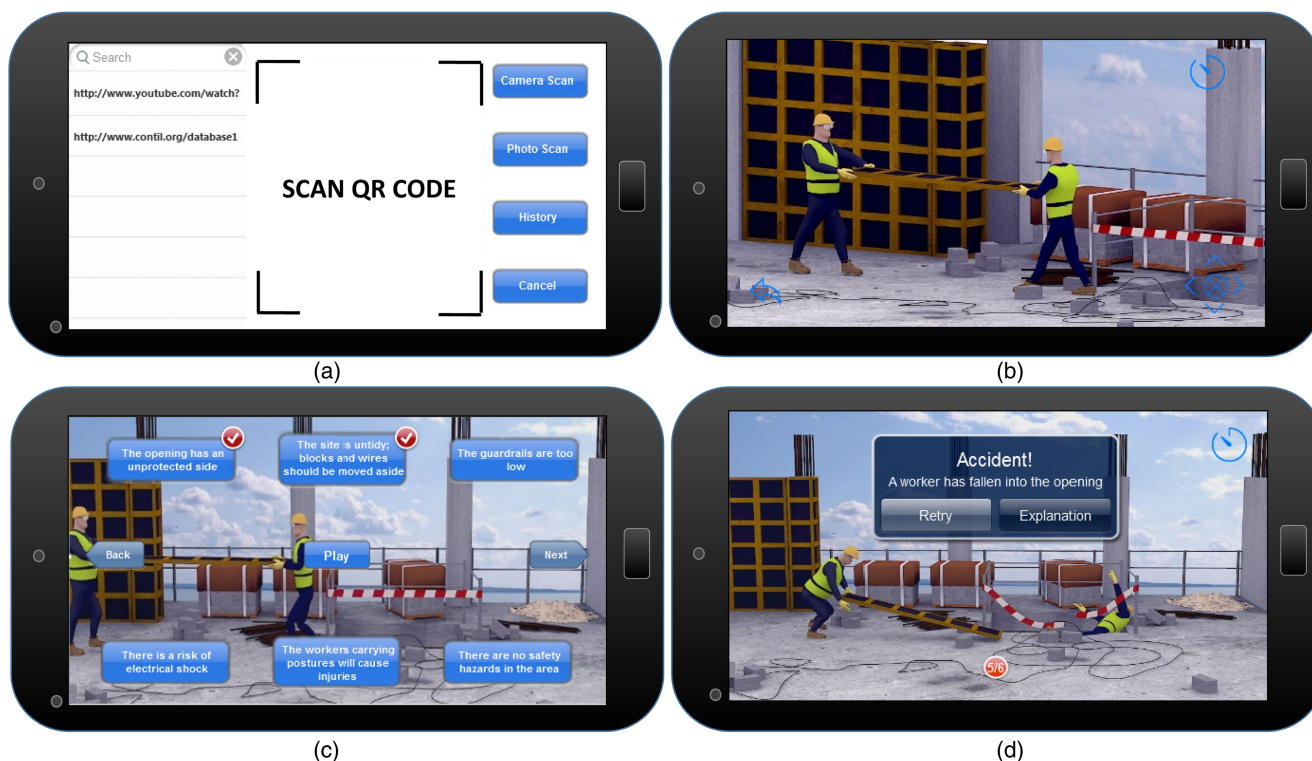
Fig. 5. Hazard inspection game process: (a) QR scanning application mobile interface; (b) virtual game scenario; (c) selecting options in hazard inspection game; (d) pop-up after accident occurs
